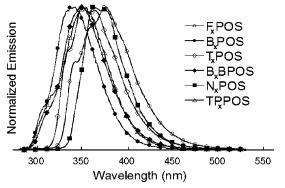
**Figure 4.** PL emission spectra (dilute THF) of Ar<sub>x</sub>OPS materials.
